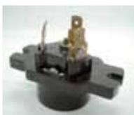
**Circle Thermal Protector (CTP) - for pumps with 1-10HP:** 3-Pole protector connects to each winding of the motor and reacts to excessive heat and amperage. Automatic reset at safe temperature to restart the motor. No motor protection circuit required in starter or control panel.
