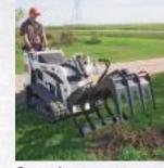
**Grapple** (Industrial, Root, Utility) Three different grapple styles: Industrial bucket grapple for demolition and removal, root grapple for sorting debris while leaving dirt behind, utility fork and grapple or bucket and grapple for light clean-up duties.
