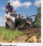
**Trencher** Handles a wide range of jobs, including trenching close to buildings. Depths down to
