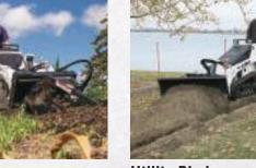
**Utility Blade** Operates as a snow blade or dozer blade. Moldboard angles up to 30 degrees.
