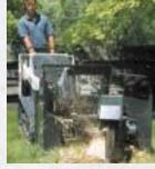
Stump Grinder Gets into tight areas and quickly grinds tree stumps into mulch.
