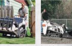
Landplane Grades, levels, transports material, breaks up hard ground and peels sod.
