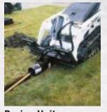
**Boring Unit** Installs utilities under driveways. sidewalks and other obstructions with minimal ground disturbance.
