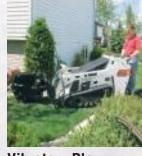
Vibratory Plow Installs flexible pipe and utilit cable 6-8 inches in the ground with minimal ground disturbance.
