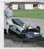
Tiller Digs and loosens soil, mixes compost and other materials into existing soil.
