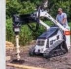
Auger Augers holes with speed and plumb-line accuracy. Bits up to 36-in, available
