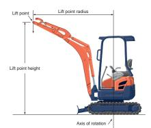
Machine with ROPS canopy and rubber crawler, without bucket
